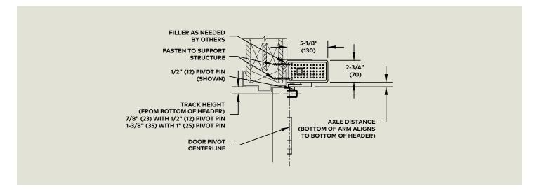
Elevation view Single pull operator Right hand door shown (left hand opposite)
